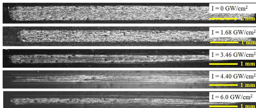
Fig. 9. Wear track on steel surfaces treated at various laser intensities.
