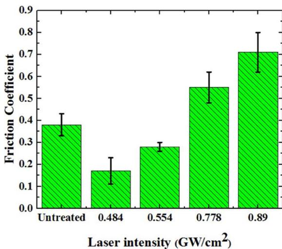
Fig. 5. Effect of laser intensity on COF.
