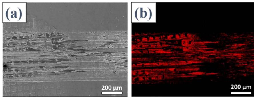
Fig. 8. Laser patterned surface after the scratching test: (a) a SEM image, and (b) EDS phase mapping of Al element. Surface micro-pattern is prepared by LSSP with a laser intensity of  $0.554 \text{ GW/cm}^2$ .
