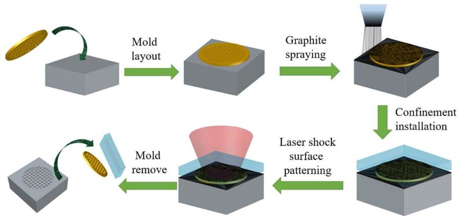
Fig. 1. A schematic illustration of indirect-LSSP process.
