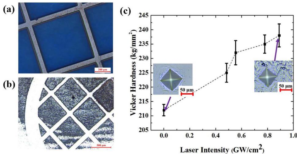
Fig. 9. (a) An optical microscope image of copper grid template with a mesh size of  $420 \mu\text{m}$ , (b) an optical microscope image of surface patterns generated by indirect-LSSP, and (c) effect of laser intensity on the hardness value of microfeature bottom area.
