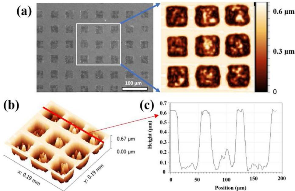
Fig. 2. (a) a SEM image and a 2-D optical image of the patterned surface, (b) a 3-D image of patterned micro-indentations, and (c) a 1-D profile of micro-indentations.
