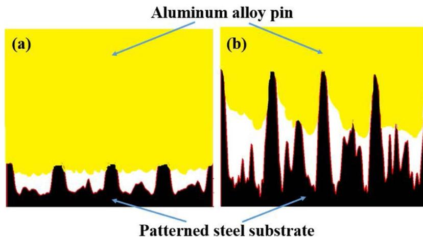
Fig. 7. Schematic illustration of contact conditions between the aluminum alloy pin and the patterned steel substrate processed by LSSP with a laser intensity of (a) 0.448 GW/cm<sup>2</sup> and (b) 0.890 GW/cm<sup>2</sup>.
