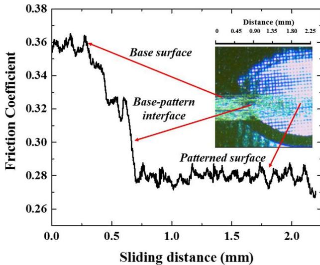
Fig. 4. Cross-over scratch tests under a dry condition: the COF on base and patterned surfaces prepared by LSSP with a laser intensity of 0.554 GW/cm<sup>2</sup>.
