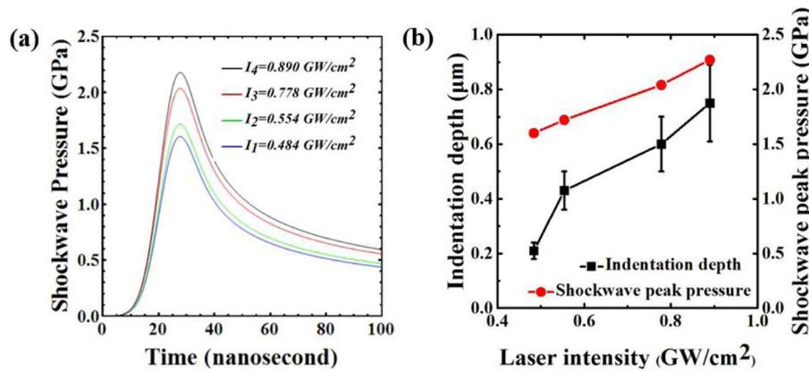
Fig. 3. (a) The temporal evolution of laser shockwave pressure as affected by the laser intensity, estimated by Fabbro's model, and (b) the indentation depth generated by indirect-LSSP at various laser intensities.
