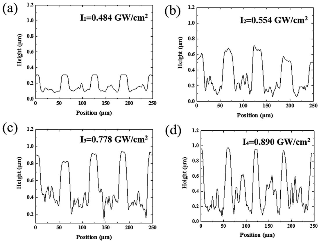
Fig. 6. Surface profiles of the patterned surfaces fabricated by LSSP with various laser intensities: (a) 0.484 GW/cm<sup>2</sup>, (b) 0.554 GW/cm<sup>2</sup>, (c) 0.778 GW/cm<sup>2</sup>, and (d) 0.890 GW/cm<sup>2</sup>.
